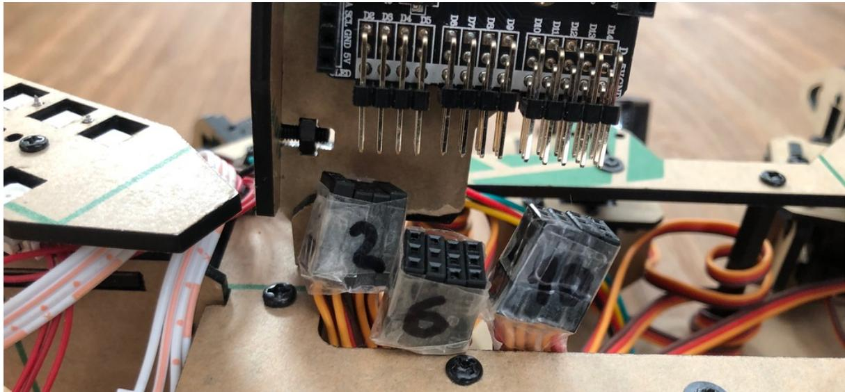
Figure 25 – AdeptPixie driver board servo pins and labeled servo connectors.
