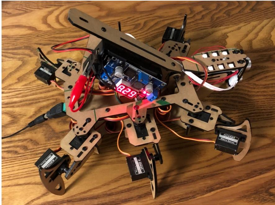
Figure 22 – An assembled robot with a built-in laboratory power supply.
